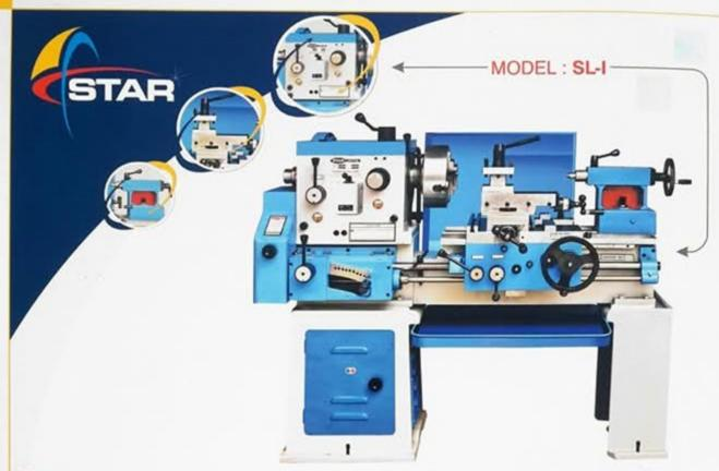
BED: Bed is a rigid casting of close grain alloy cast iron of Brinell Hardness 200 ± 10 with webbed inverted vees to withstand heavy loads with minimum of vibration & deformation. All bearing surfaces are hard & ground. High tensile induction hardened slide v-ways are also available on requirement.
